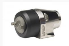
The Ecco 75AP is designed for applications in small and narrow areas. It has a 70% reduced inner space for the paint, which reduces the paint consumption, especially when many colour changes are made. Angles of paint channels have been optimized for best possible cleaning effect. Well-known technology has been used in air caps and nozzles in combination with optimal design of the gun body. The result is a very compact unit with highest possible performance.
