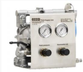
Pump panel for your tailor made pump unit. The pump panel includes a diaphragm pump Ecco Flow AL15, bracket, pressure gauge and regulators. Fits all Ecco low pressure spray guns and hoses.
