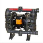
Ecco Flow CT15 is a lubrication free diaphragm pump with non freeze and non stalling air system. The pump has a modular design, is easy to maintain and has high air efficiency. The CT15 is a conductive plastic pump with diaphragms in PTFE, suitable for many pumpable fluids in temperature range 0-66°C.
