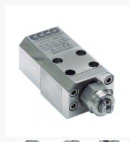
Ecco 380A is an automatic airless gun, designed to fit most types of high-pressure applications in automated production lines. Valve seat and needle tip are made in tungsten carbide for long durability. The gun can be changed in less than two minutes without any loss of mechanical precision or performance.
